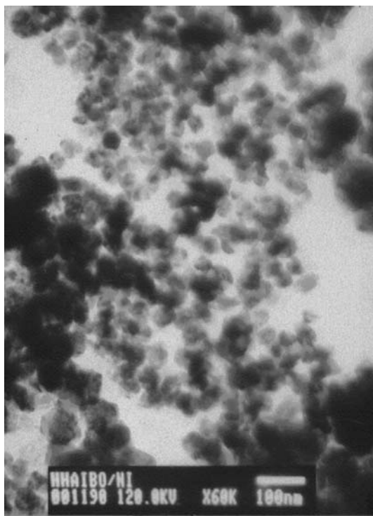
Figure 10 Transmission electron micrograph of the sample precipitated by the reduction of \text{Ni}^{2+} with hydrazine in solution. Reaction conditions: T = 298 \text{ K} , [\text{Ni}^{2+}]_0 = 0.68 \text{ mol/l} , [\text{N}_2\text{H}_4]_0 = 3.26 \text{ mol/l} and m(\text{NaOH}) = 2.5 \text{ g} . BET area = 18 \text{ m}^2/\text{g} .
